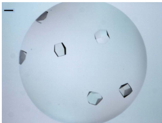
Figure 2 Typical crystals of native SHARPIN obtained using the two-dimensional grid seeding method with 4 M sodium formate as precipitant. The crystallization drop (0.6 \mu\text{l} ) contained 3.9 \text{mg ml}^{-1} SHARPIN (final concentration) with the addition of 45 \text{nl} native seed solution in 4 M sodium formate. The scale bar represents 0.1 mm.
